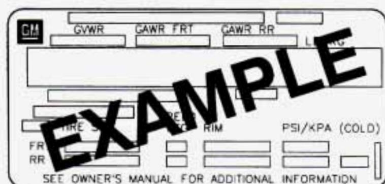
The Certification/Tire label is found on the rear edge of the driver's door. The label shows the size of your original tires and the inflation pressures needed to obtain the gross weight capacity of your vehicle. This is called the GVWR (Gross Vehicle Weight Rating). The GVWR includes the weight of the vehicle, all occupants, fuel and cargo.
