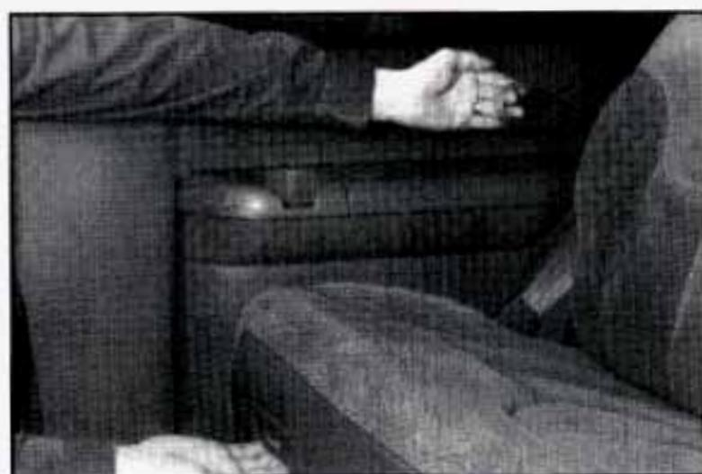
When you release the seat cushion, the seatback is automatically released. Pull the loop on the seatback forward and fold the seatback into the seat cushion.
