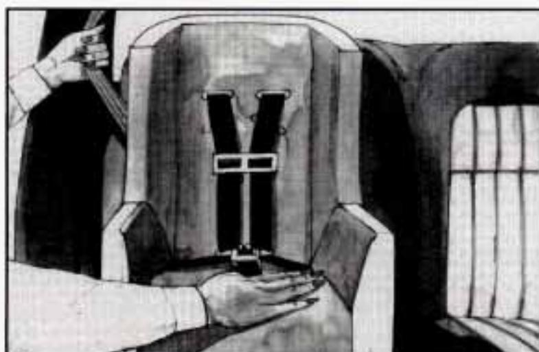
5. To tighten the belt, pull up on the shoulder belt while you push down on the child restraint.
