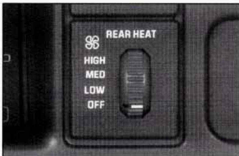
If you have a rear heater (without rear air conditioning), the control switch is located on the instrument panel.
