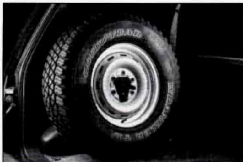
First open the tire cover, if you have one. Turn the wing nut counterclockwise and take it, and the adapter, off the bolt. Take the tire out of the vehicle and remove the tire cover.
