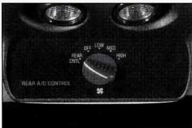
To operate the rear system using the front control, just turn the knob to the blower position you want.
