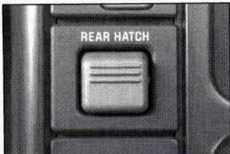
The electric hatch release button lets you release the tailgate glass. To release the glass, press the top of the switch button.
