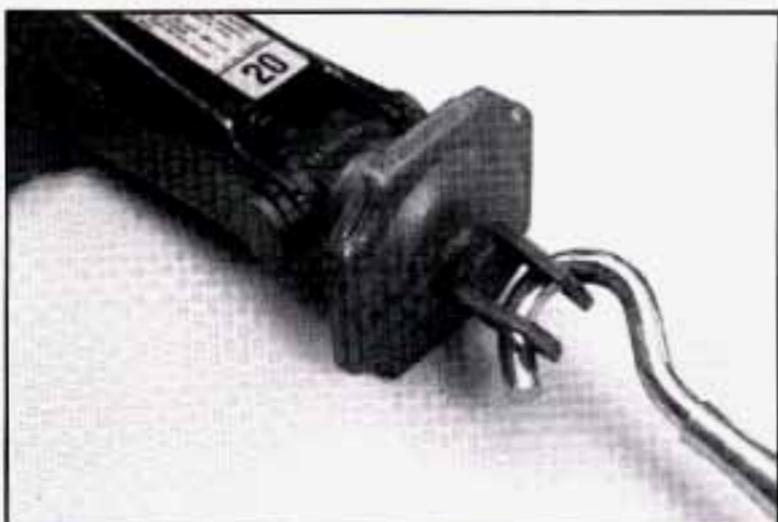
Attach the jack handle (and jack handle extension, if needed) to the jack. One side of the ratchet has an UP marking. The other side has a DOWN marking.
