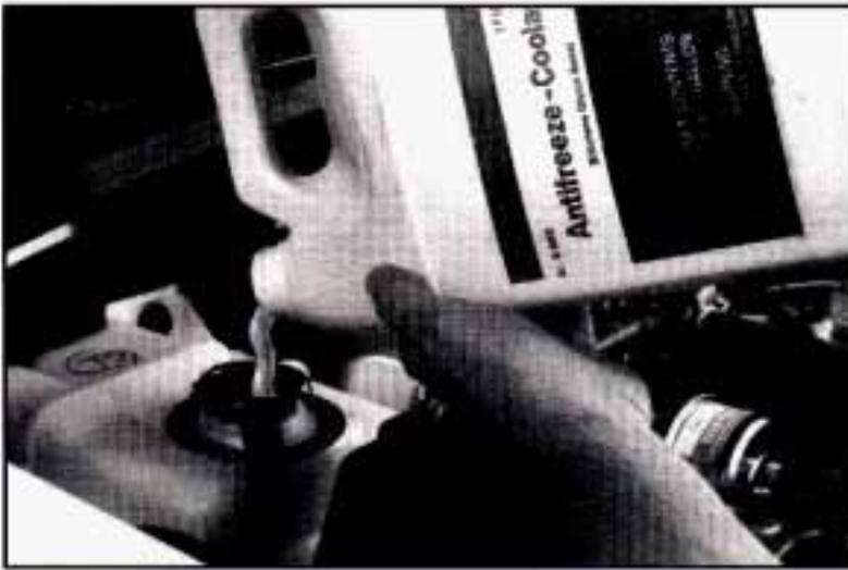
7. Then fill the coolant surge tank with the proper mix, up to the COLD mark.
