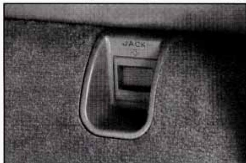
To open the jack cover on 4-door utility models, push the cover latches down and remove the cover.
