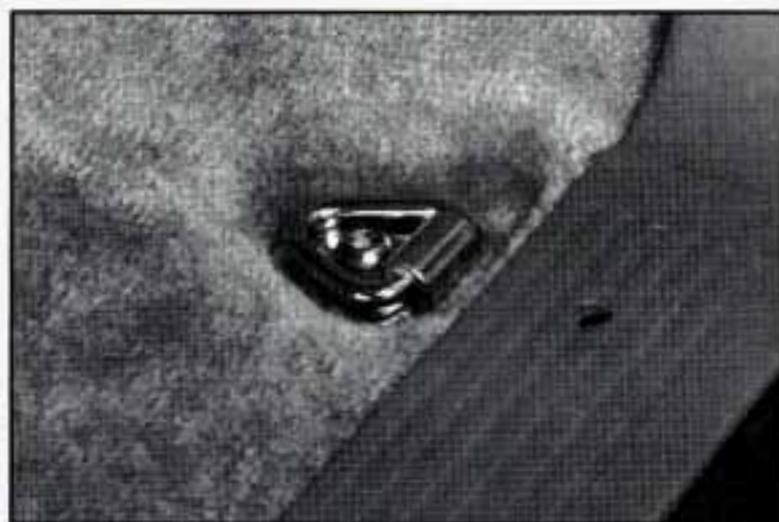
There are cargo tie downs in the rear cargo area that allow you to strap cargo in and keep it from moving inside the vehicle.
