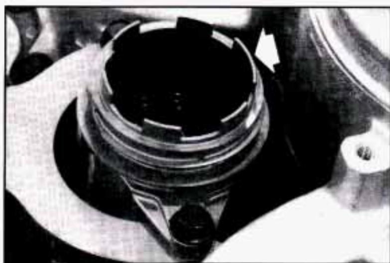
6. Line up the widest slot in the top of the new element with the widest key on then top of the filter head. Push the element in until the mating surfaces touch.
