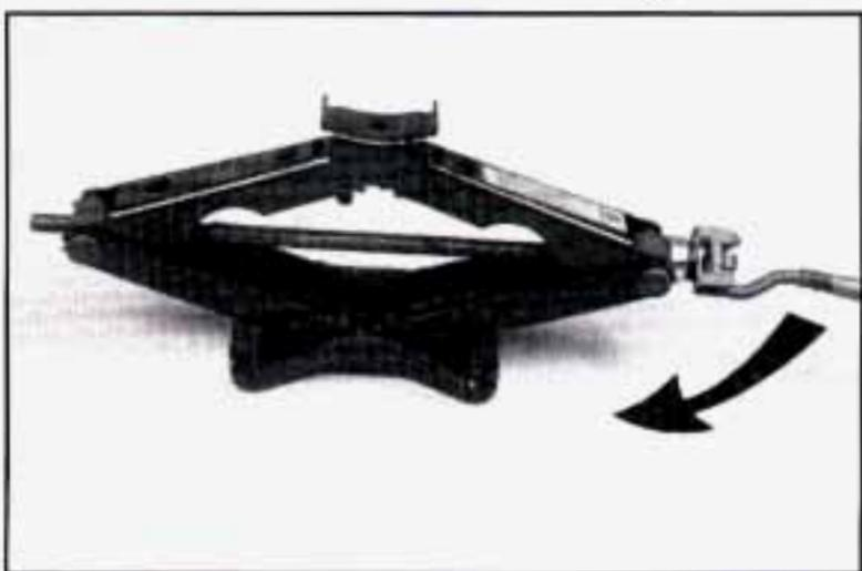
With the UP marking on the ratchet facing you, rotate the ratchet clockwise. That will lift the jack head a little.
