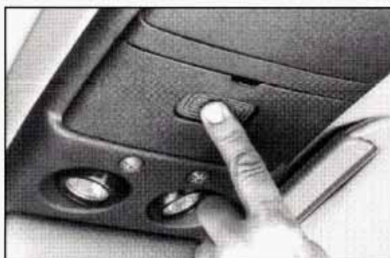
Now, with the compartment door closed, push the button marked **PUSH** again to make sure the garage door opener operates properly.
