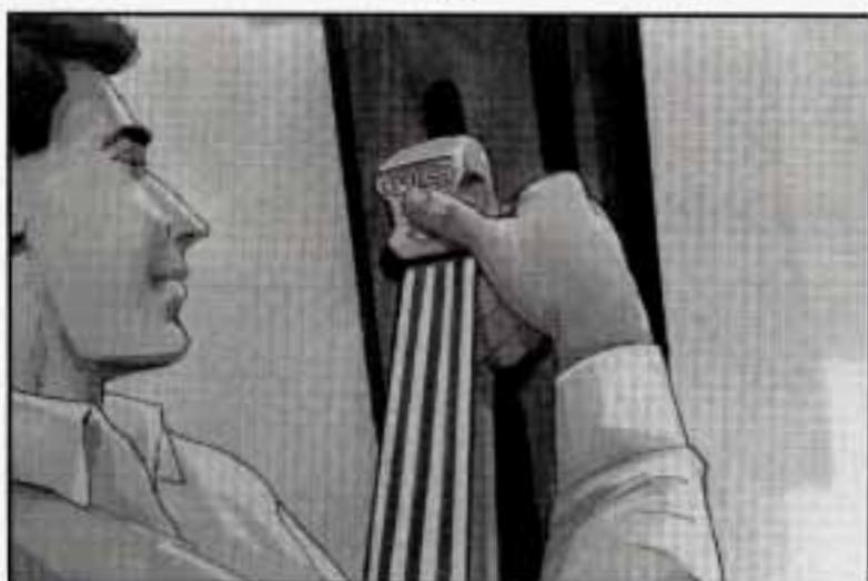
To move it down, push in at the word **PRESS** and move the height adjuster to the desired position. You can move the adjuster up just by pushing up on the shoulder belt guide. After you move the adjuster to where you want it, try to move it down without pushing in to make sure it has locked into position.
