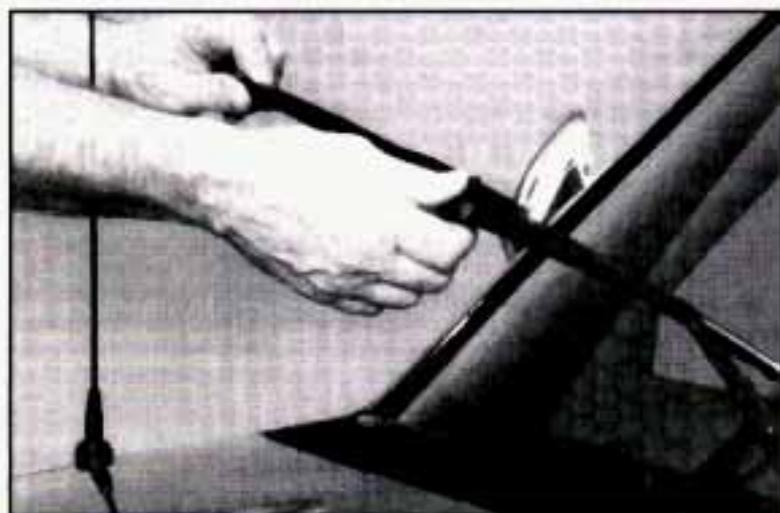
To replace your windshield wiper blade inserts, lift the wiper arm and rotate the blade until it is facing away from the windshield.
