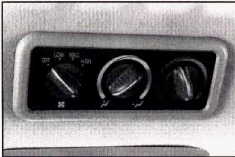
The rear control works just like the front control. It will allow second seat passengers to adjust the controls as they desire.
