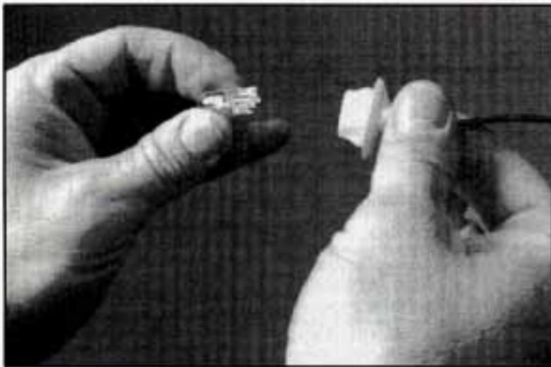
3. Pull the bulb straight out of the socket.
