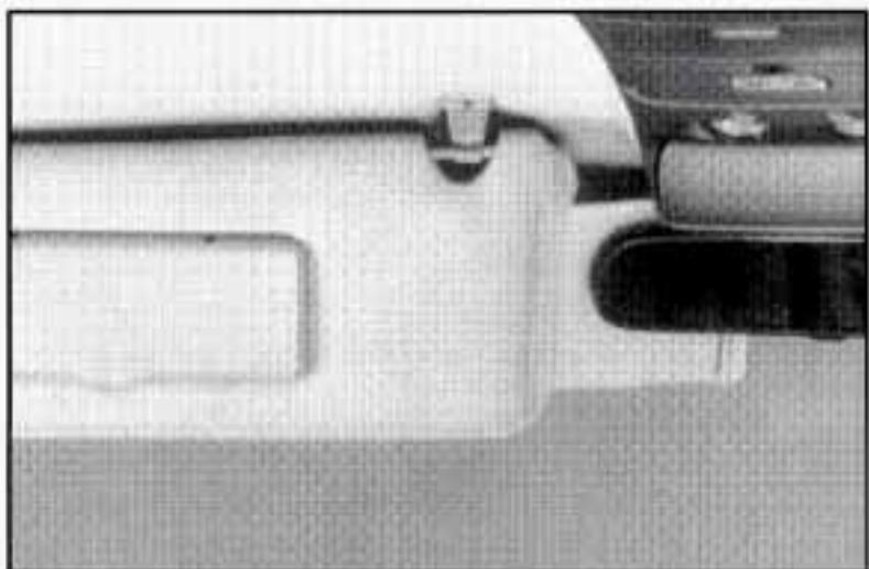
Some visors have an extender on the inside edge. When the visor is down, pull the extender out for extra glare coverage at the front or side.
