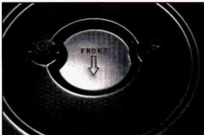
To avoid the possibility of un-filtered air being drawn into the engine, make sure the air cleaner cover is on straight and the wing nuts are properly tightened. If there is an arrow on the air cleaner cover, it should point to the front of the engine.
