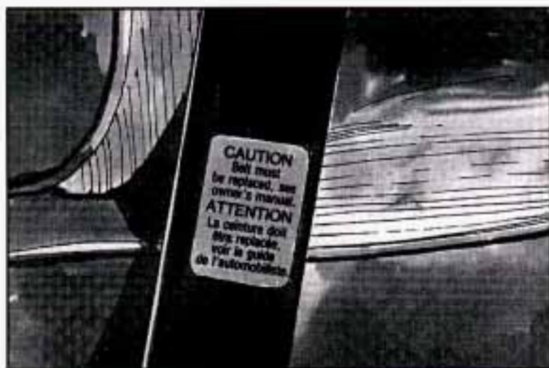
If belts are cut or damaged, replace them. Collision damage also may mean you will need to have safety belt or seat parts repaired or replaced. New parts and repairs may be necessary even if the belt wasn't being used at the time of the collision.
