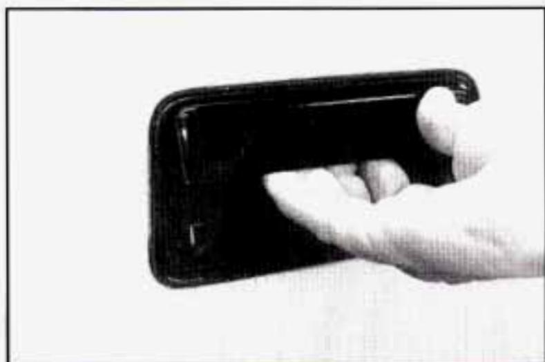
To open the passenger's side door, pull up on the handle and pull the door open.
