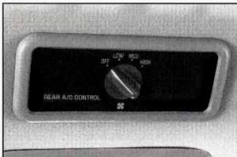
To use the rear control, first turn the front control knob to REAR CNTL. Then, the rear control can be used to increase and decrease the air flow.
