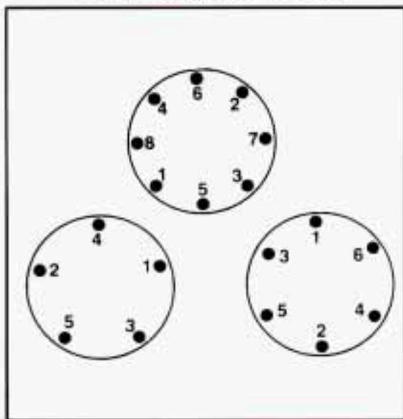
Tighten the nuts firmly in a criss-cross sequence as shown. Rotate the wheel wrench clockwise.
