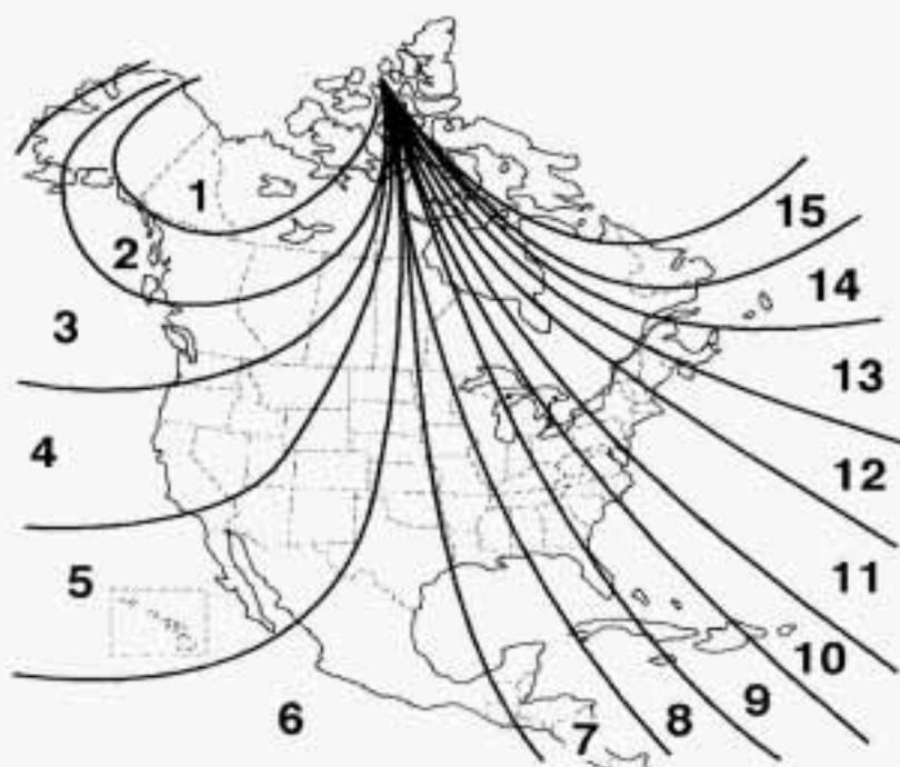
3. Press and hold the CAL switch until the new zone number appears in the display. After you release the switch, the display will show a compass direction within a few seconds.
