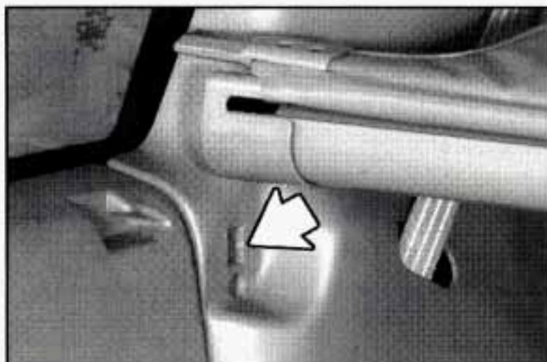
Push the shade holder toward the passenger side of the vehicle and place the tab in the driver's side trim panel slot. Make sure the tab goes all the way in the slot.
