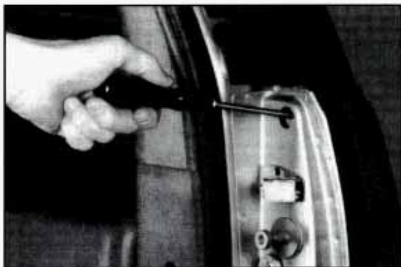
3. Remove the two rear lamp assembly screws inside the fender and pull out the lamp assembly. You may want to use a magnetic screwdriver when removing the screws.
