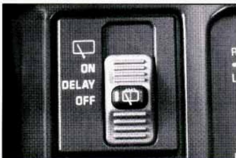
The rear window wiper/washer switch is on your instrument panel, to the passenger side of the gage cluster.
