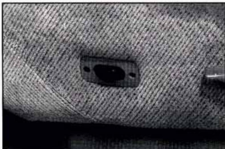
To adjust the power lumbar, press the front of the lumbar switch at the side of the seat. Press the front of the switch to increase lumbar support. Press the rear of the switch to decrease lumbar support.
