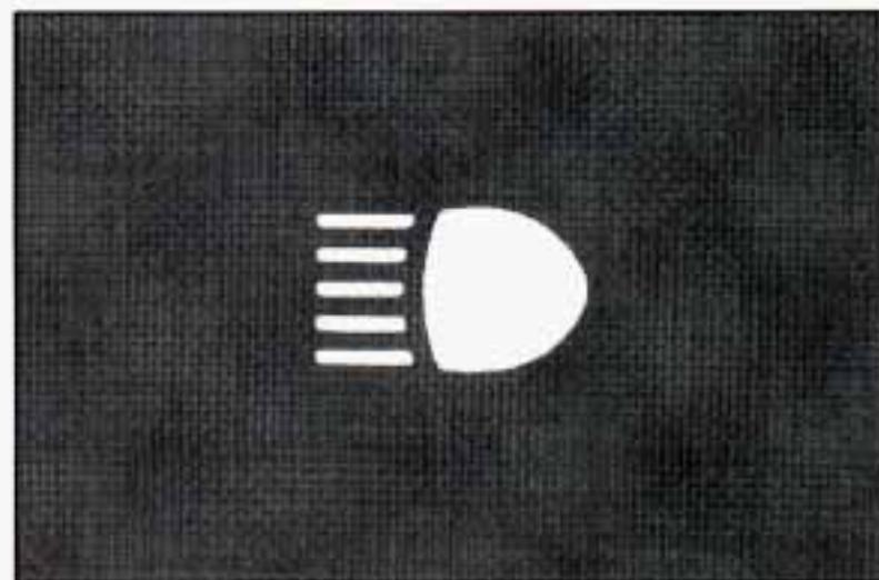
The blue high beam indicator is on whenever you use your high beam headlamps. For more details about high beams, see “Headlamp High–Low Beam” earlier in this section.
