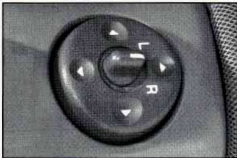
Select the mirror you want to move by moving the center of the switch, located on the driver's door armrest, to R (right) or L (left).
