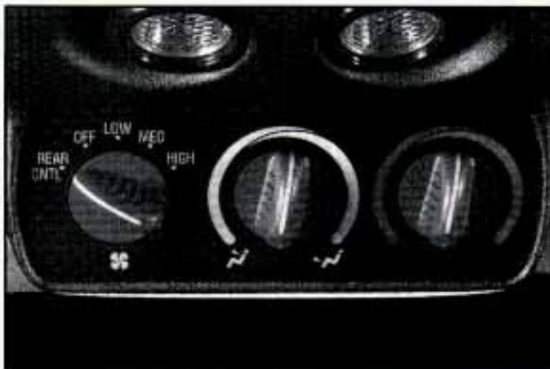
To adjust the air temperature, turn the temperature knob on the right side of the control panel.
