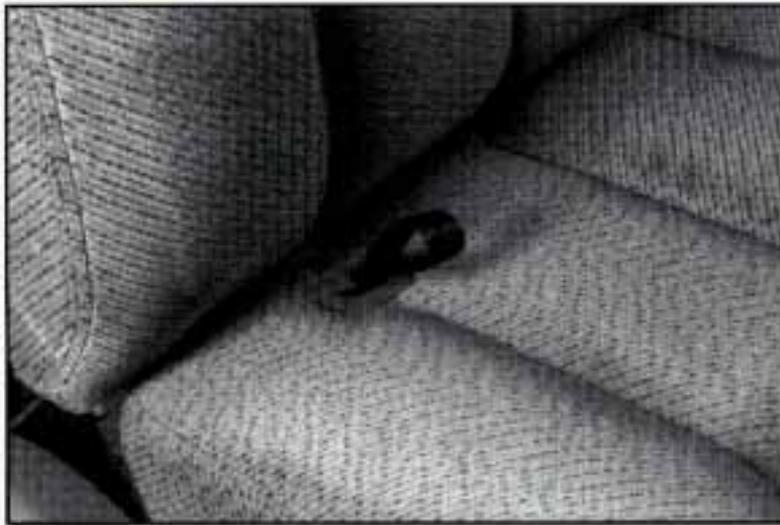
To fold the seat, pull up on the strap loop at the rear of the seat cushion.
